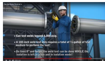
Step 11 (Perform hydrotest at required pressure)
