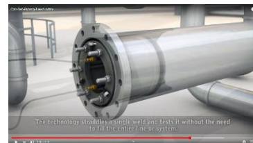
Step 10 (Shift weld tester to required position)
