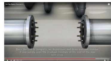
Step 12 (Completed of test & depressurized)
