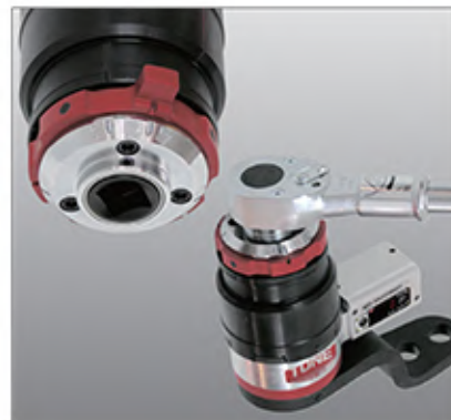
Combined of anti-wind-up clutch and ratchet handle improves workability and protects operator from spring back force of the gears.
