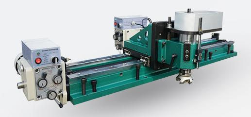
MRY1200 Line Milling Machine is suitable for repairing straight/flat profiles or surfaces. The machine can be rigidly locked onto the surface (to be machined) using bolts. It is compact, lightweight, and allows easy installation and removal with two persons. This portable milling machine is designed for a wide range of on-site milling activities, such as keyway milling, mounting surfaces milling, tubesheet gasket seat milling etc.
